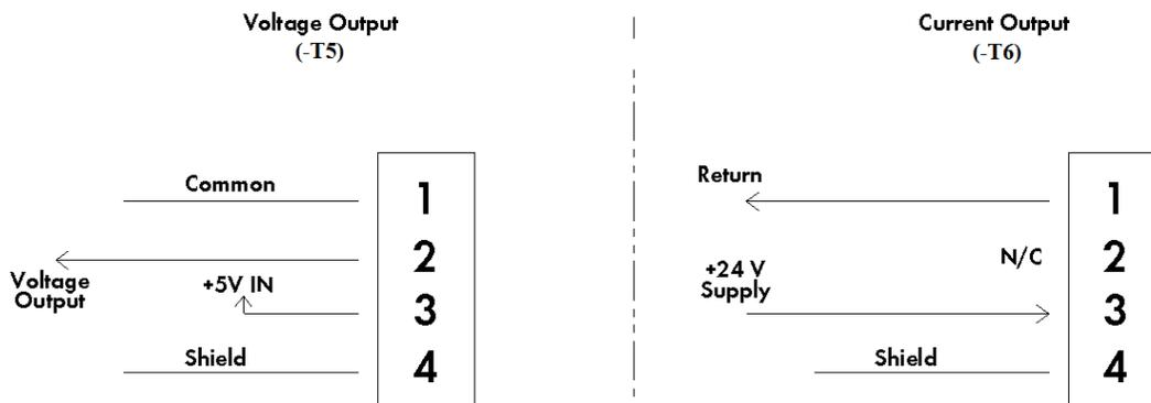
Voltage input is 5VDC  $\pm$  5% for 0.5-4.5VDC output devices.
